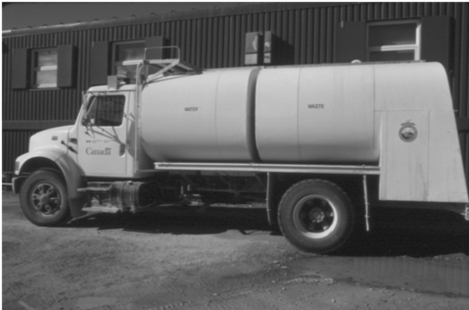
Fig. 11.23 The sewage and water truck that services the hamlet of Resolute Bay (Nunavut). The truck delivers water from Char Lake to the water tanks of local residents, but also pumps out their sewage and gray water holding tanks and transports to the local dump for land disposal. Hopefully the two tanks are never confused!
