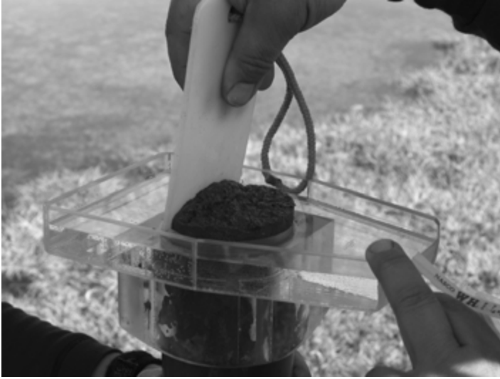
Fig. 4.6 Sectioning a surface, gravity sediment core at high resolution (e.g., 0.25 cm intervals), using a Glew (1988) vertical extruder. Photograph taken by M. Douglas.
