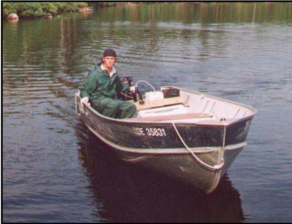
*A field assistant adds estrogen to the surface waters of Lake 260 using an automated pump.*
